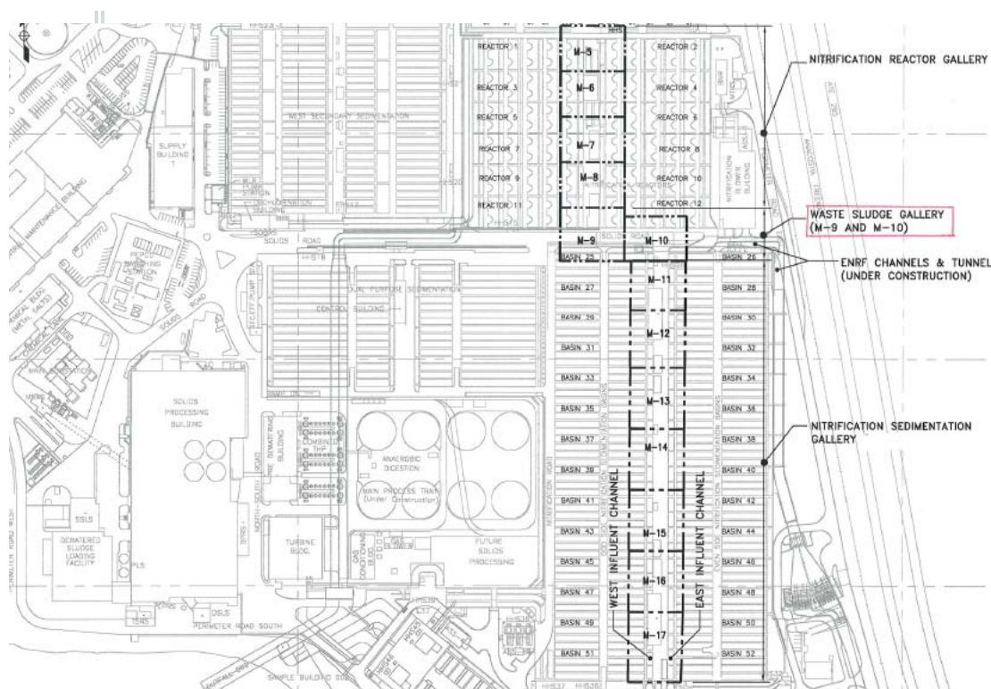
Figure 3. Plan view of Nit RAS Pipeline
